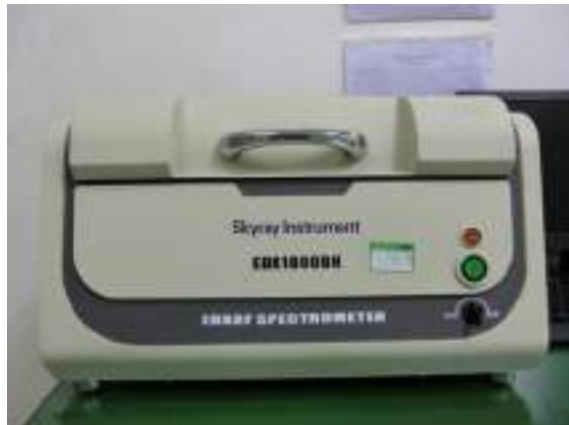
RoHS - XRF螢光光譜儀 RoHS – XRF fluorescent spectroscope
