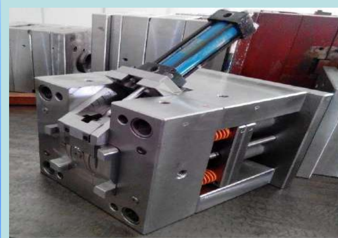
Arc Core Pulling
