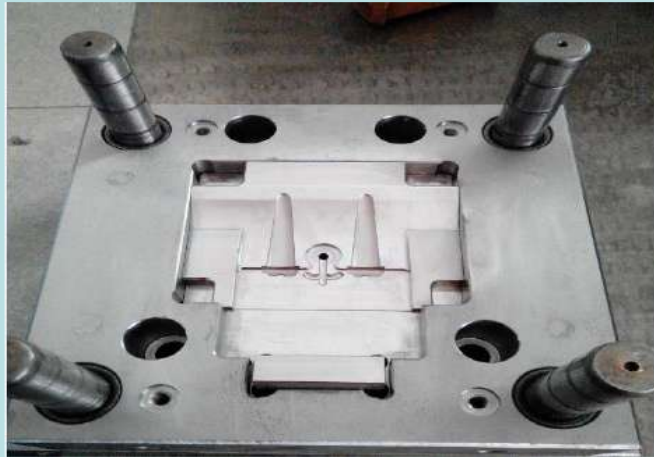
Arc Core Pulling
